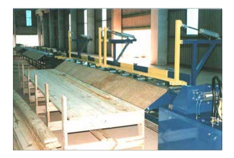
A belt driven roller conveyor fitted with pneumatically operated kickers to eject reject timber as determined by the Strength Testing Machine. The conveyor is also fitted with a guide arrangement designed to keep the timber upright while passing to Full Length Marker but is automatically removed prior to a reject being ejected.
