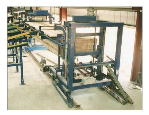
Successive boards are transferred to the Auto Stacker which accommodates 5 boards in width and up to 25 layers in depth (normally set to 20).
