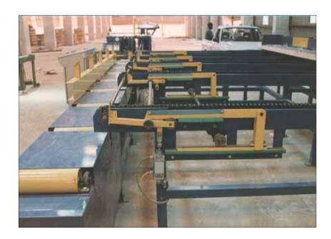
This apparatus is a four or five strand chain which employs a width adjustable hold and release mechanism, designed to hold back all timber allowing only the first piece to be released to the infeed conveyor. The profile of the feeder together with the infeed guide are responsible for turning the timber on edge ready for grading.
