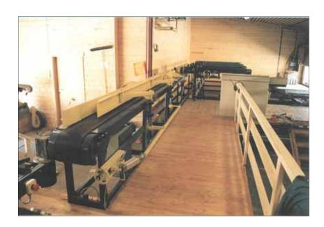
A heavy duty belt conveyor equipped with a moving guide mechanism designed to keep the timber upright until it has entered the strength testing machine. On entry to the machine the guide will automatically be removed to prevent interference with the grading process.
