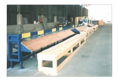
This conveyor is a belt driven roller conveyor fitted with pneumatically operated kickers to give two separate timber collection stations. The kick signals are issued from the central control console and can be selected to accommodate any permutation of the four grades available at the Strength Testing
